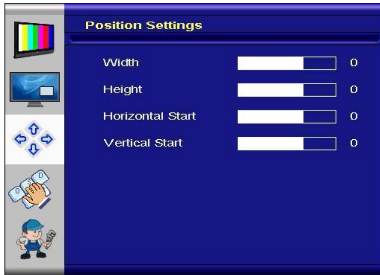
Figure 9.4.a: "Position Settings" menu for video mode of HDMI, S-Video, composite and component inputs.
