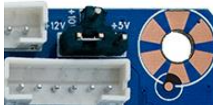
Figure 3 Jumper for voltage selection
