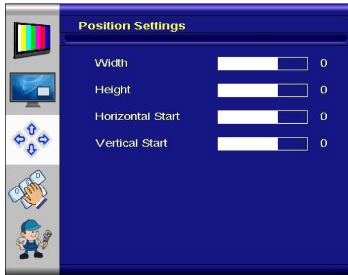
Figure 7.3.a: “Position Settings” menu for video mode of HDMI, S-Video, composite and component inputs.
