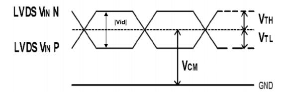
Figure 4.1 LVDS DC characteristics
