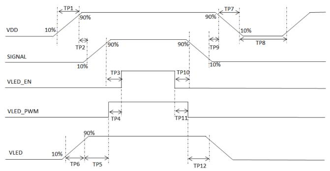
Figure 5.2 Interface power on/off sequence
