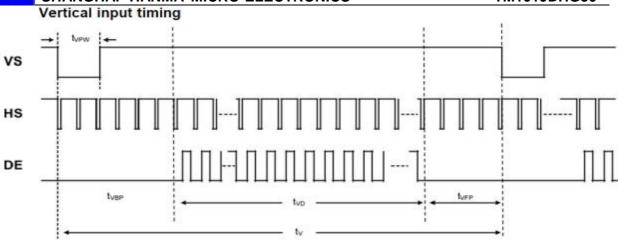
Figure 5.2 Input signal data timing
