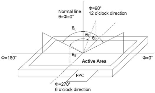
Fig. 1 Definition of viewing angle
