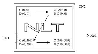
Figure 1. Normal scan (DPS: Low or Open)
