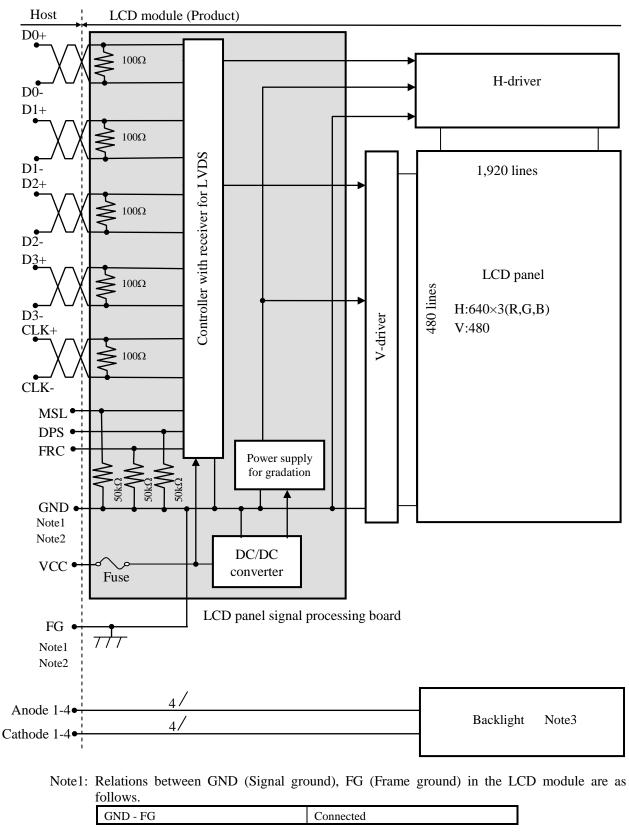
Note2: GND and FG must be connected to customer equipment's ground, and it is recommended that these grounds be connected together in customer equipment.
