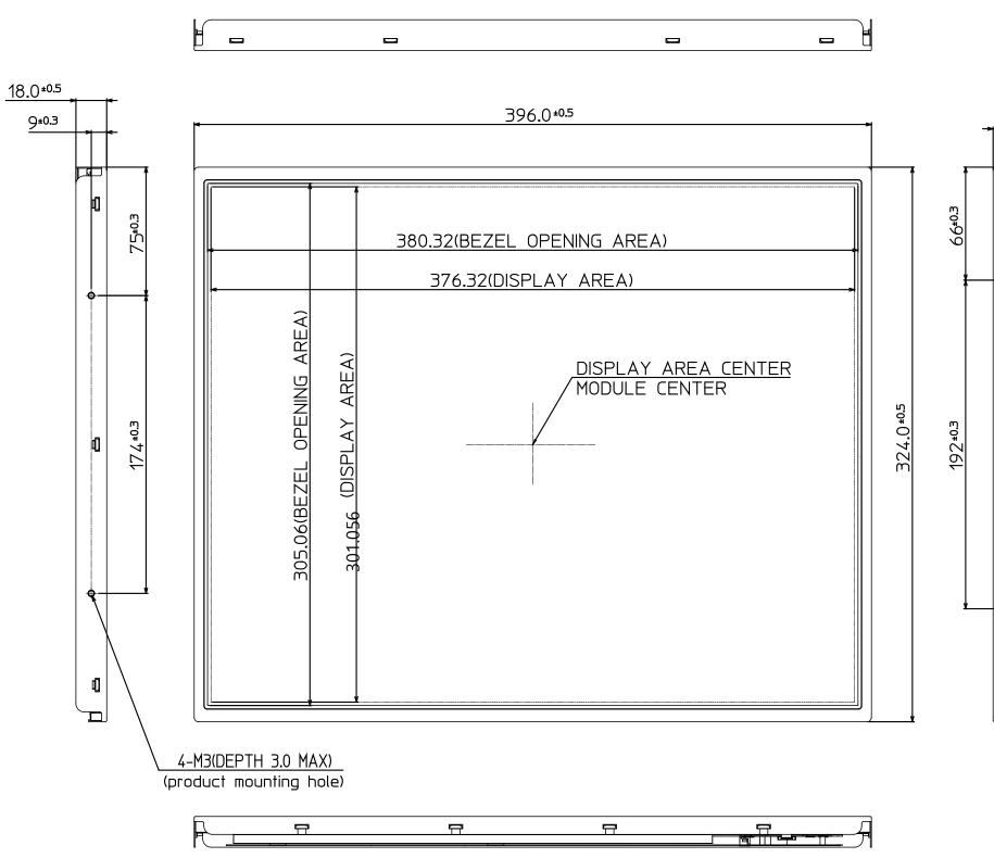
Note1: The torque for product mounting screws must never exceed 0.67N·m. And the length of product mounting screws from surface of plate (product side) must be  $\leq 3.0$  mm.
