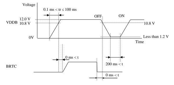
Note1: The backlight should be turned on within the valid period of LVDS signals, in order to avoid unstable data display.
