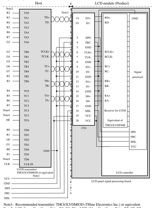
4.5.4 Connection between receiver and transmitter for LVDS
