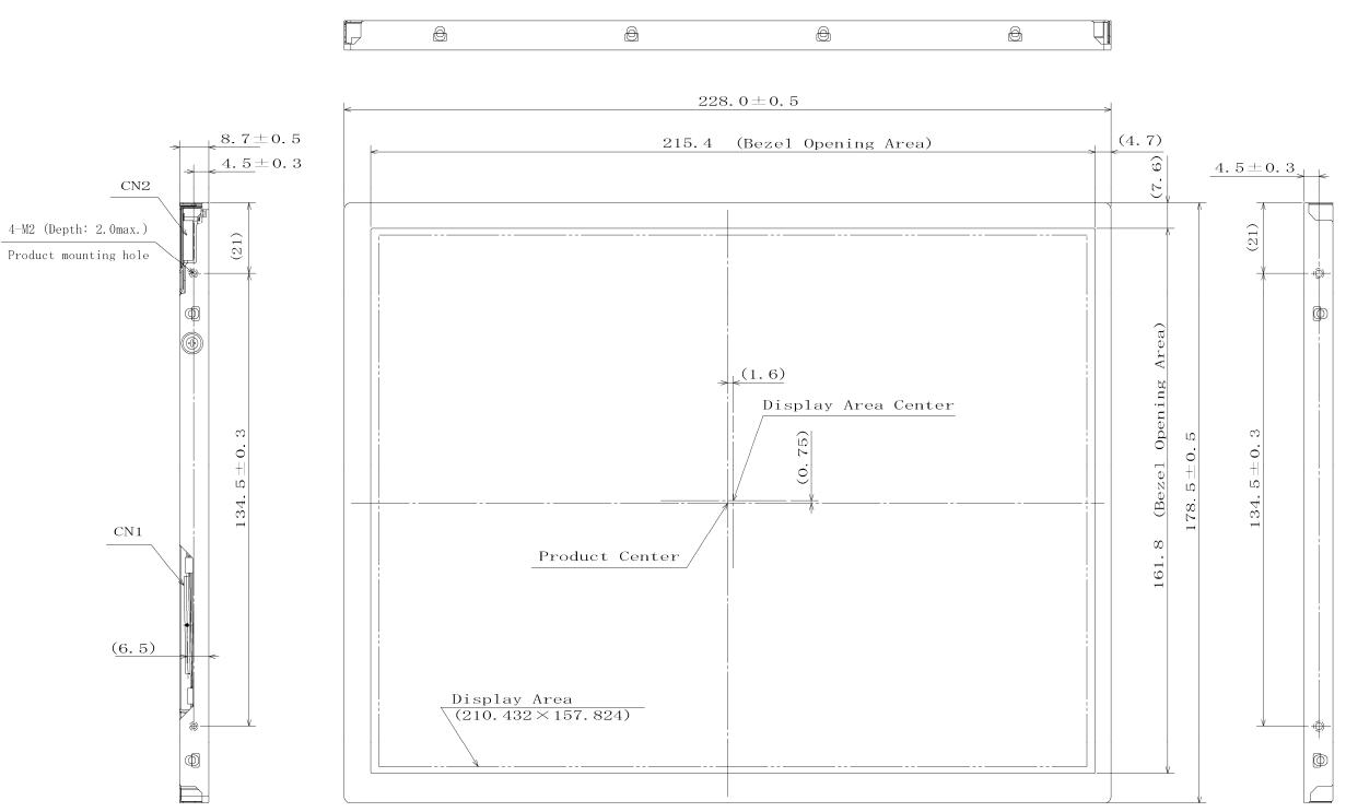
Note1: The values in parentheses are for reference. Note2: The torque for product mounting screws must never exceed 0.147 N·m.
