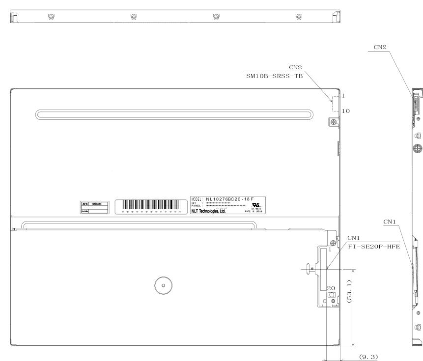
Note1: The values in parentheses are for reference. Note2: The torque for product mounting screws must never exceed 0.147 N·m.
