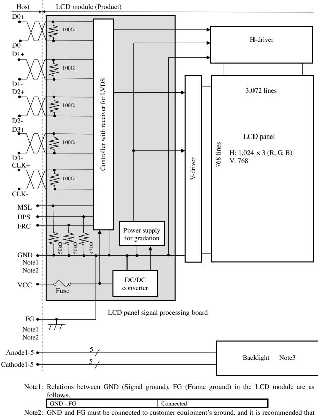
Note2: GND and FG must be connected to customer equipment's ground, and it is recommended that these grounds be connected together in customer equipment.
