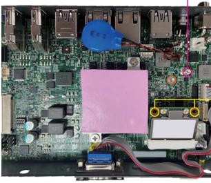
Module holes for tightening the bracket with the bundled screws. Note that the module in this image is not screwed to the bracket.
