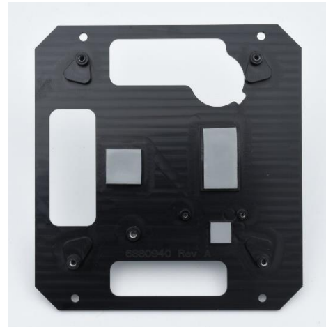
Heat spreader inner surface
