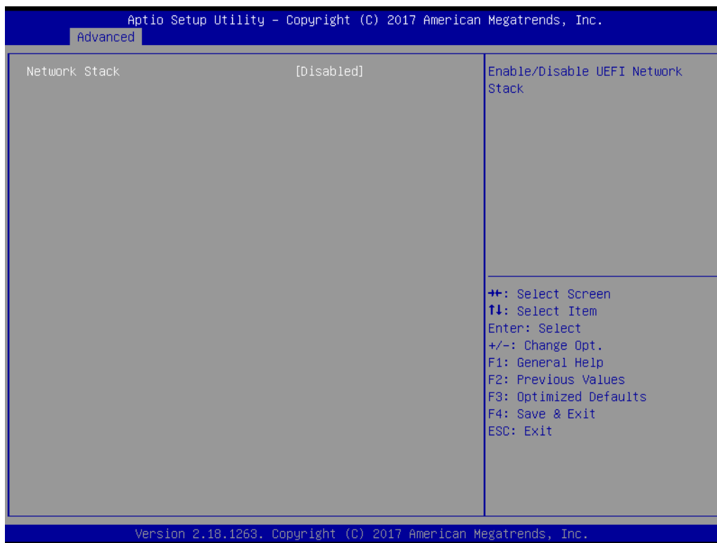
Figure 3.14 Network Stack Configuration
