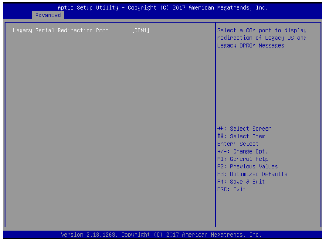
Figure 3.15 Legacy Console Redirection Settings
